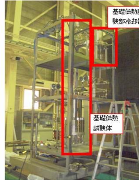
Supercritical water loop (JAEA)
